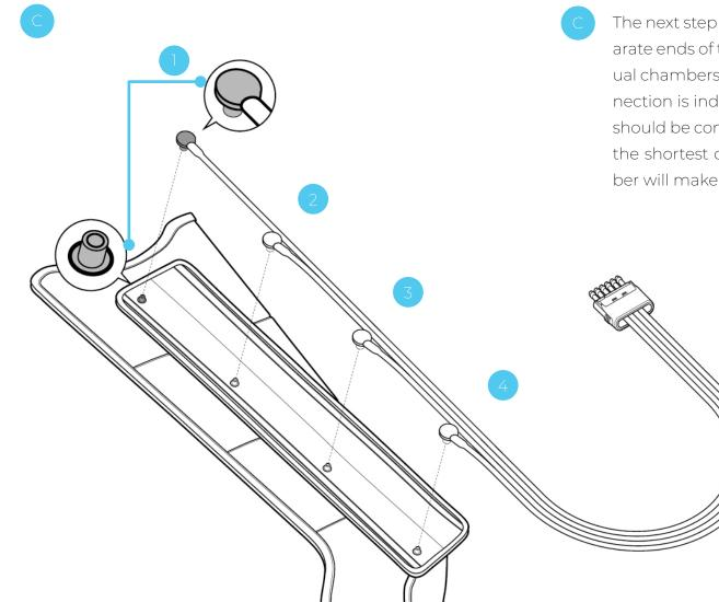
The next step is connecting the air duct to the cuff. The separate ends of the air duct should be clipped into the individual chambers of the cuff with correct order. The proper connection is indicated by a dark gray plug. The separate ends should be connected in following order: from the longest to the shortest one. Correctly plugged end in the cuff chamber will make a characteristic click.
