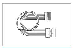
Double splitter (long - 150 cm) for 8-chamber devices
